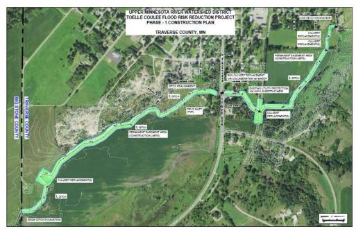
**Toelle Coulee - Phase One** The goal of the Toelle Coulee Project – Flood Damage Reduction is to provide 100-year flood protection to the rural community of Browns Valley. Toelle Coulee Phase I consisted of the west ditch improvements and was completed in 2020 and inspections were completed in 2024.
