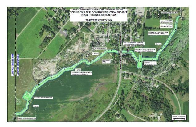
The goal of the Toelle Coulee Project – Flood Damage Reduction is to provide 100-year flood protection to the rural community of Browns Valley. There are five elements to the Toelle Coulee Project, Phase I consisted of the west ditch improvements and was completed in 2020 and inspections were completed in 2021. Routine maintenance checks to track volunteer tree growth were completed.
