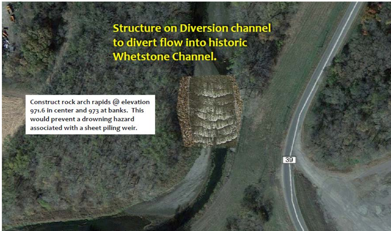
Figure 8: Concept Design of Whetstone River Diversion Structure Preferred by Minnesota Department of Natural Resources
